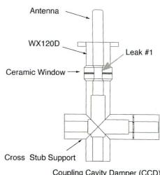
Coupling Cavity Damper (CCD)
