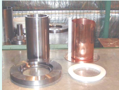
Mandrel, Die and Fabricated Cu-pipe
