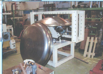
End Plate of Vacuum Vessel for Cryostat made by Spinning
