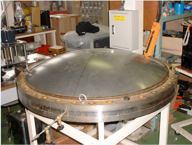
\phi 1200, 1.5 t SUS 316L End Shell for Vacuum Vessel
