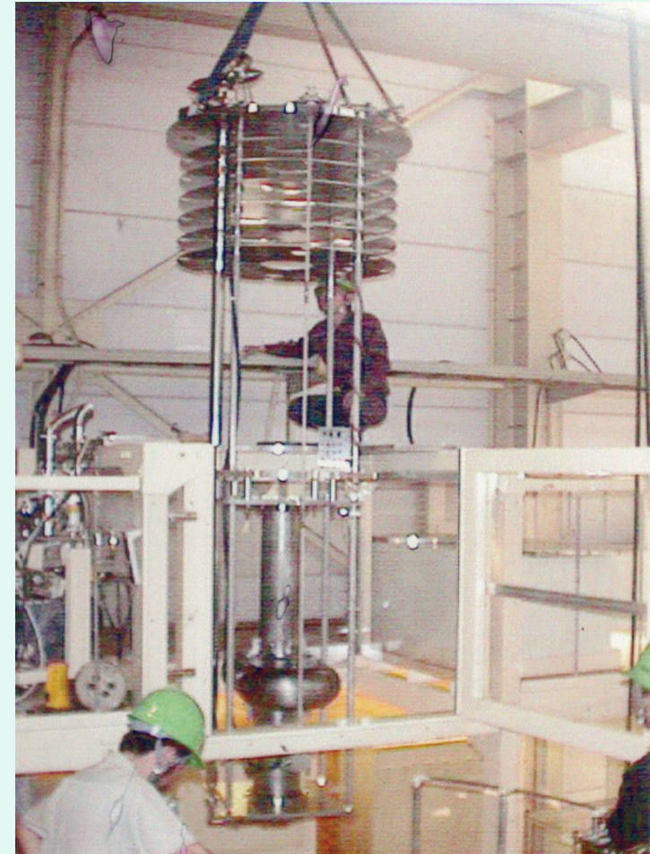
The crab cavity is taken out from clean room to install into the vertical cryostat.
