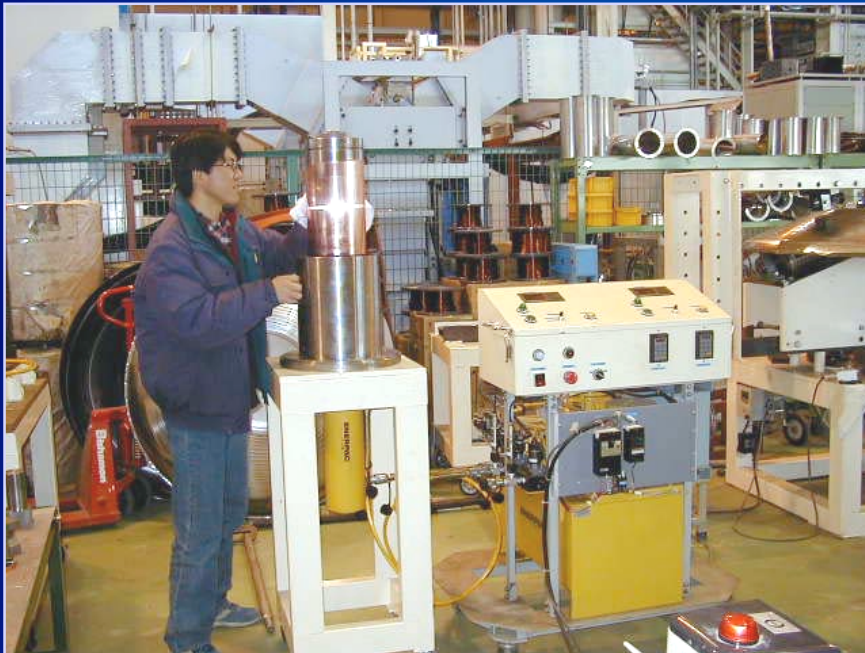
Drawing Bench: Capacity 30 tons
