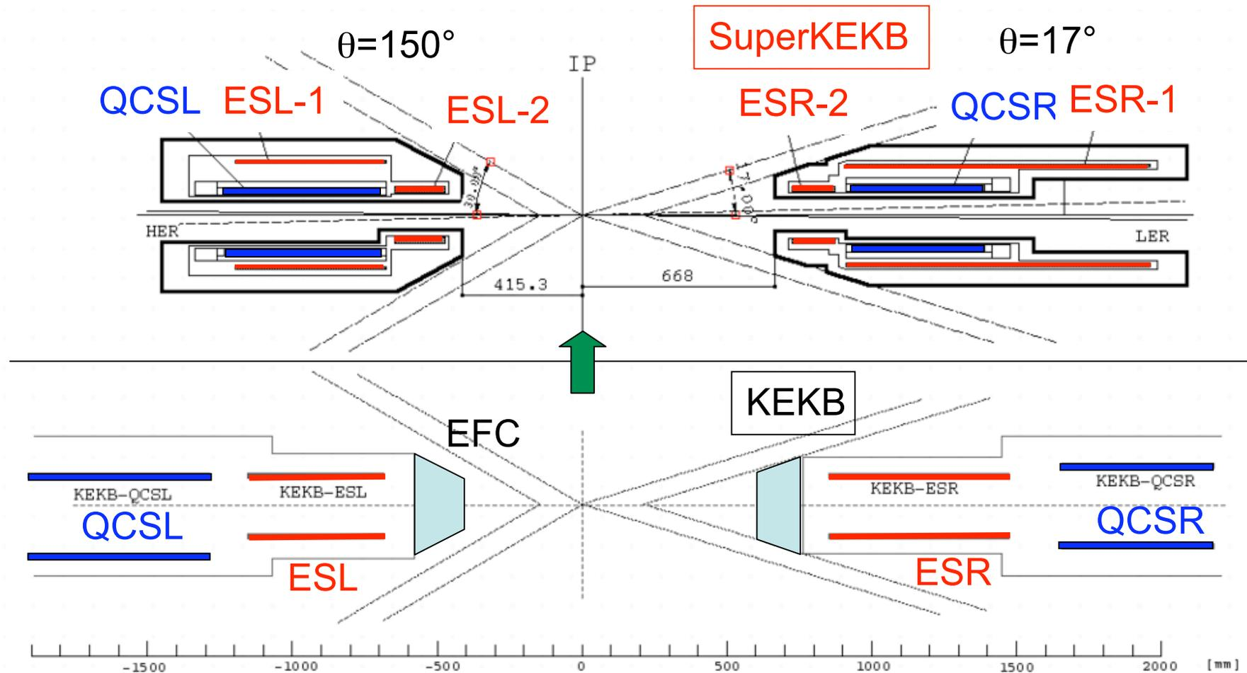
Move QCS closer to IP and compensation solenoid (ES) is divided into two parts; one is overlaid with QCS, the other is in front of QCS.
