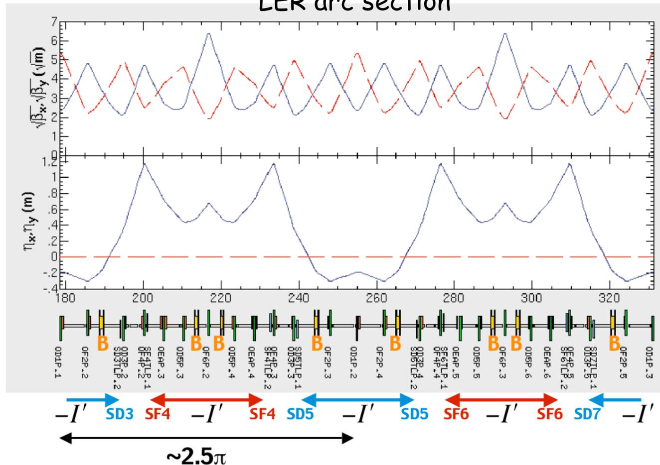
Two sextupole magnets in a pair are connected with -I' transformer.
