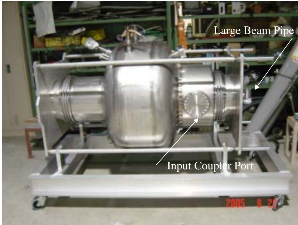
Jacket Type Helium Vessel
