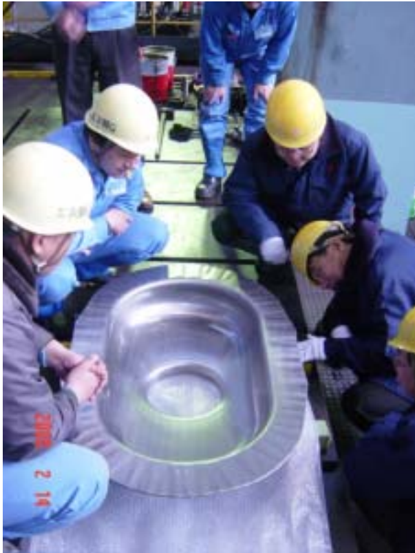
Forming of 4 Half-Cells for Crab Cavity for LER and HER
