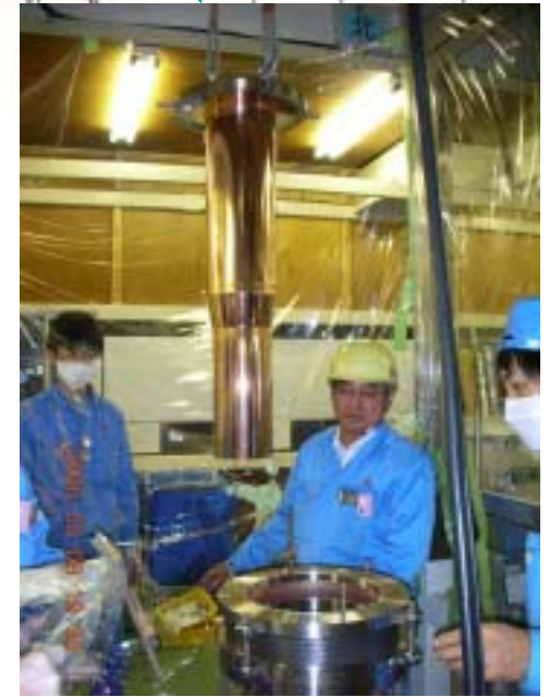
Copper Plating SUS Inner Conductor Cooled by Water
