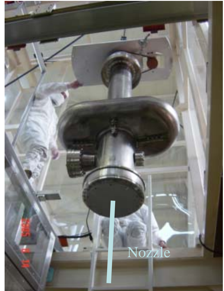
High Pressure Water Rinsing by 80 bar Ultra-Pure water
