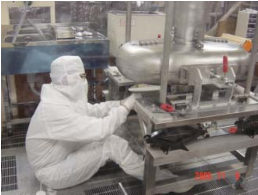
Set Flanges of Beam Pipes and Ports in Class 100 Clean Room
