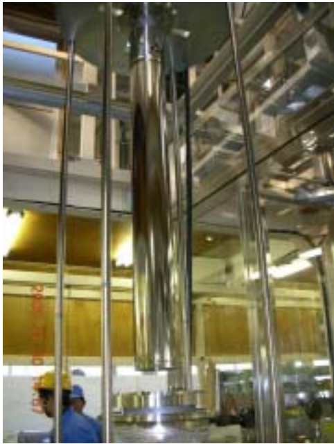
Nb-Coaxial Coupler Cooled by Liq. Helium
