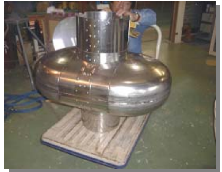
Jacket Type Magnetic Shield
