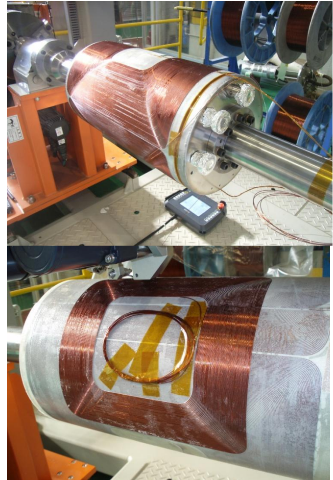
Automatic winding of the skew and the normal dipole correctors by Toshiba. 11
