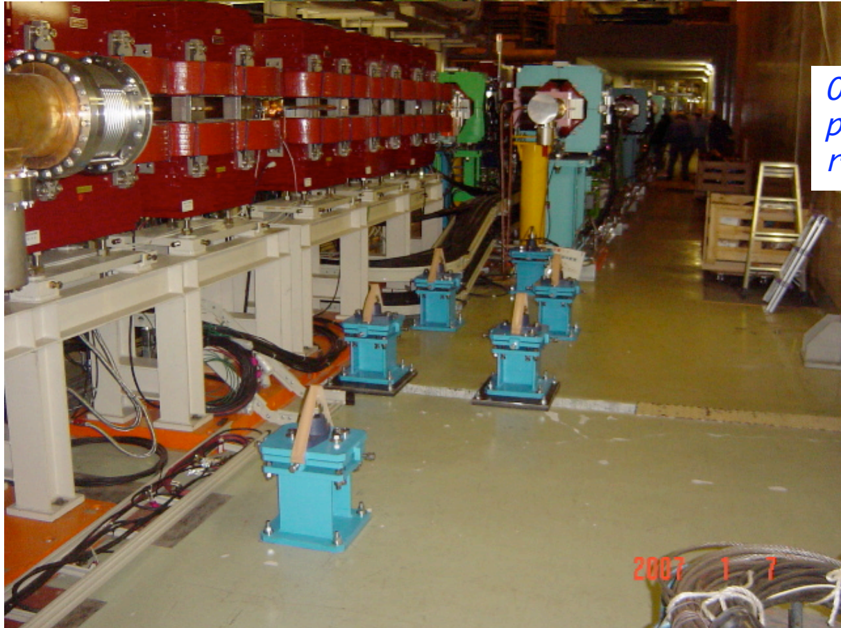
Support legs: 4 for weight support/ 2 for flatness
