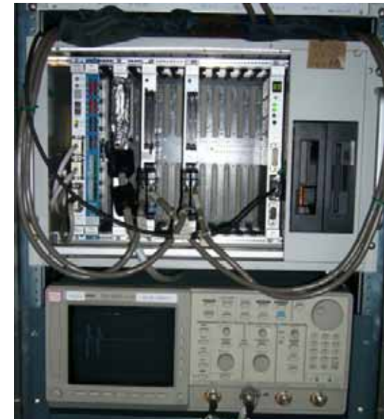
BPM DAQ system (VME + Oscilloscope with GPIB)
