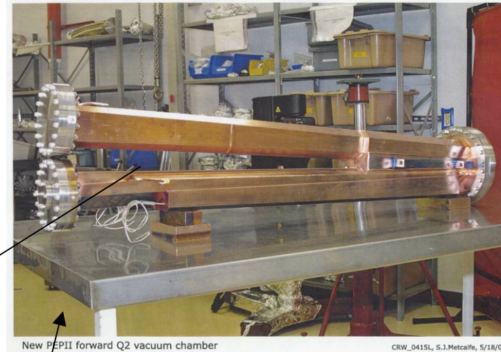
New PEP-II forward Q2 vacuum chamber CRW_0415L, S.J.Metcalf, 5/18/02
