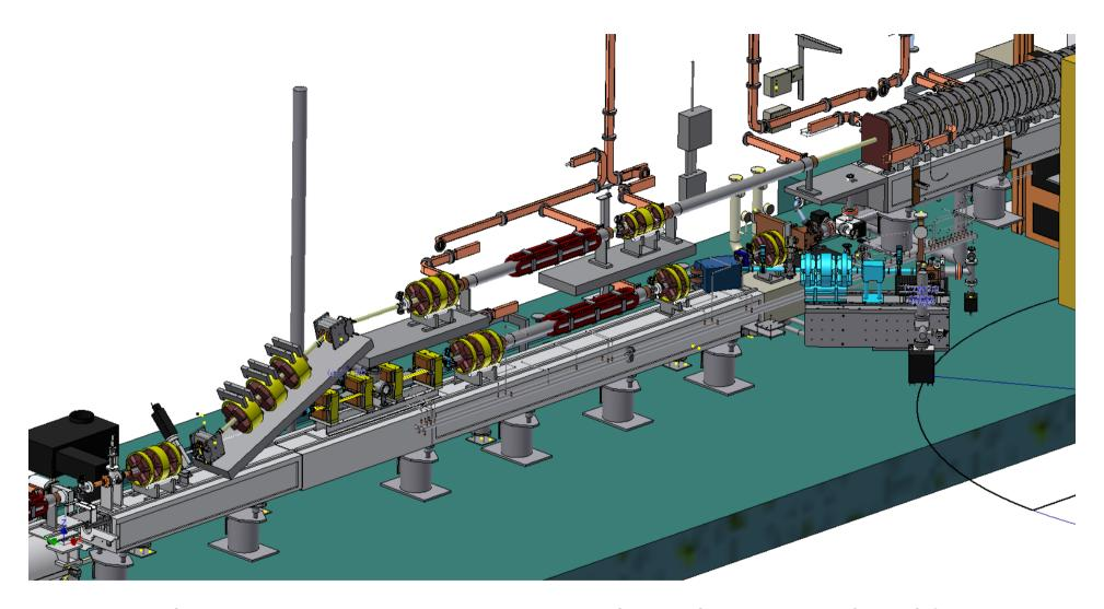
This came as a surprise ... a new beamline using the old thermionic gun and now two quasi-travelling wave guns
