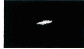
Fig.5 Beam profile after deconvolution process, scale is same as in Fig.4.
