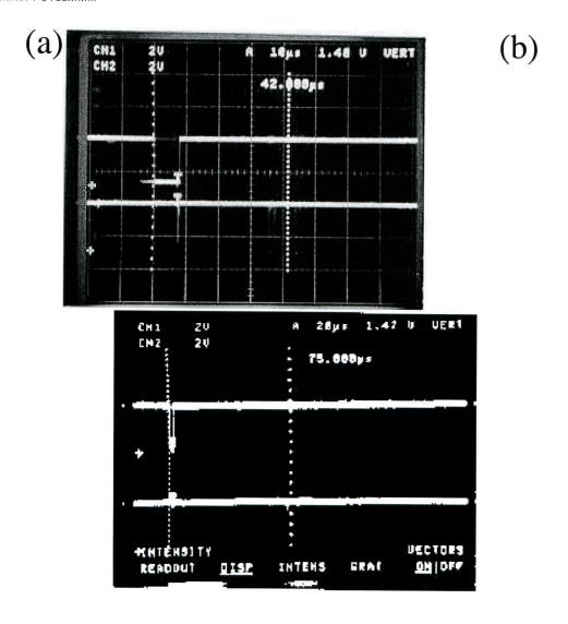
Response to an external interrupt on PPC(a) and 68040(b)
