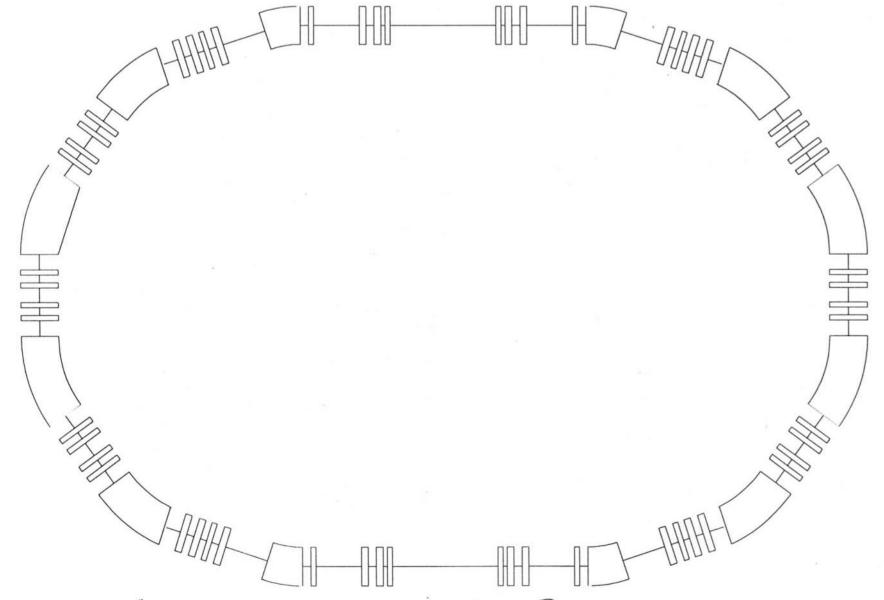
Special consideration on Lattice Design \* make the structure more tight. using half B for dispersion suppressor. \* diffrent phose advance at H & V plain.
