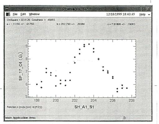
Tolerances needed to keep the high-current beam hitting the positron target at more than 90% of the best tuned intensity (9.4 nC/bunch at that time)
