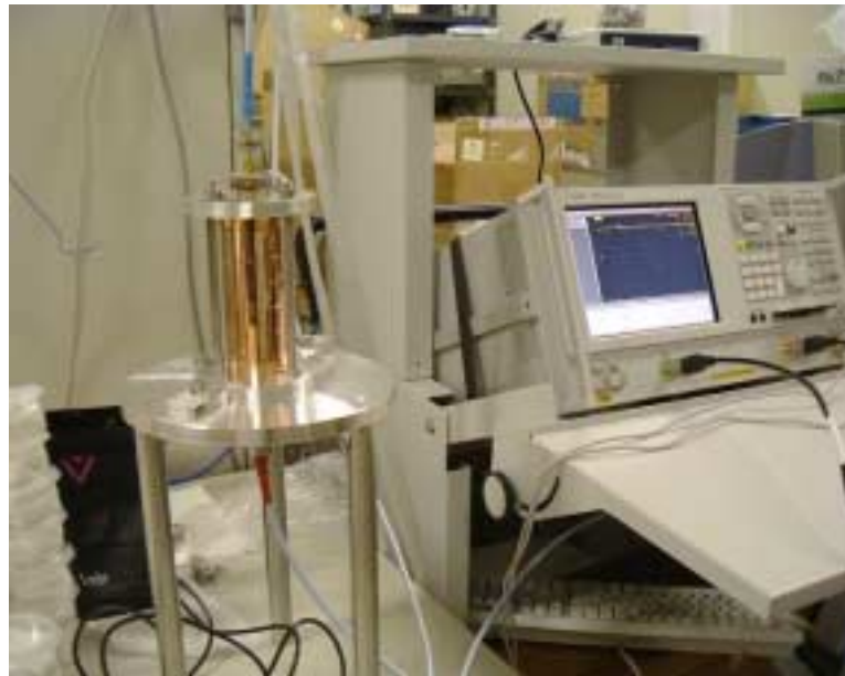
Left photo shows the standard cavity to give the standard frequency for other manufactured Cavity.
