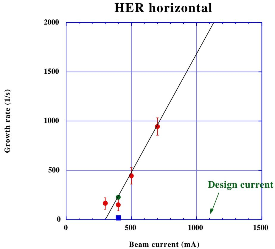
Damping time of 0.5ms is necessary for suppressing the CBI at the design current of 1.1A.
