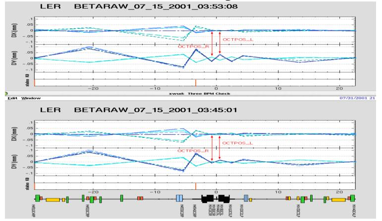
Correlation error at IR was calculated from the difference in the singlekick orbits in HER by the three- BPM correlation method (upper: electron beam; lower: both beams)
