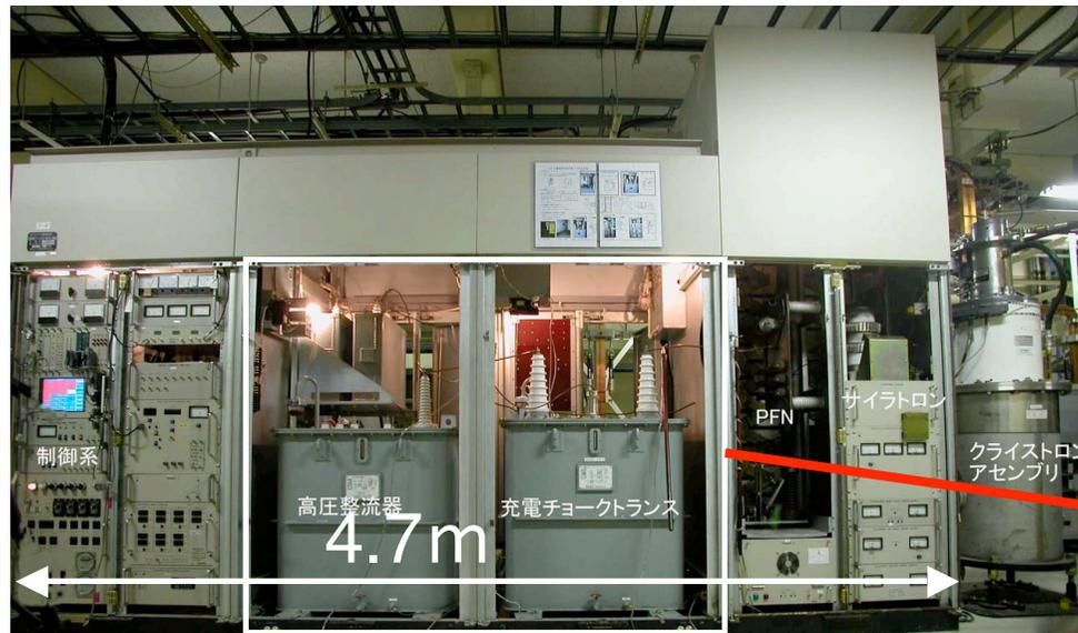
S-band modulator & klystron
