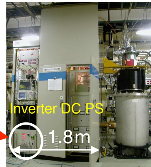
C-band modulator & klystron
