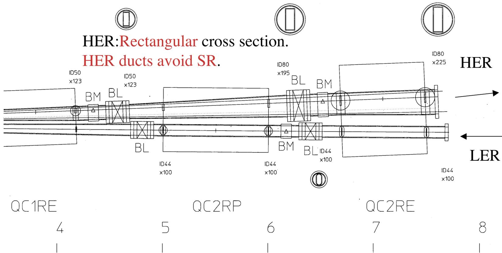
BM:Beam Position Monitor, BL:Bellows
