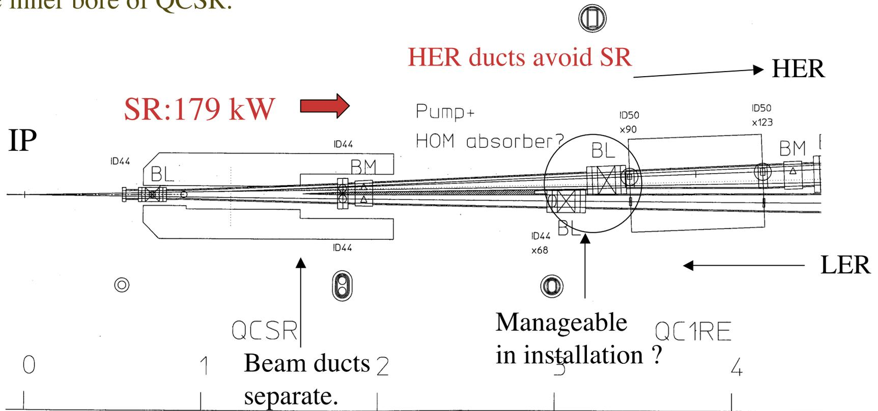
BM:Beam Position Monitor, BL:Bellows
