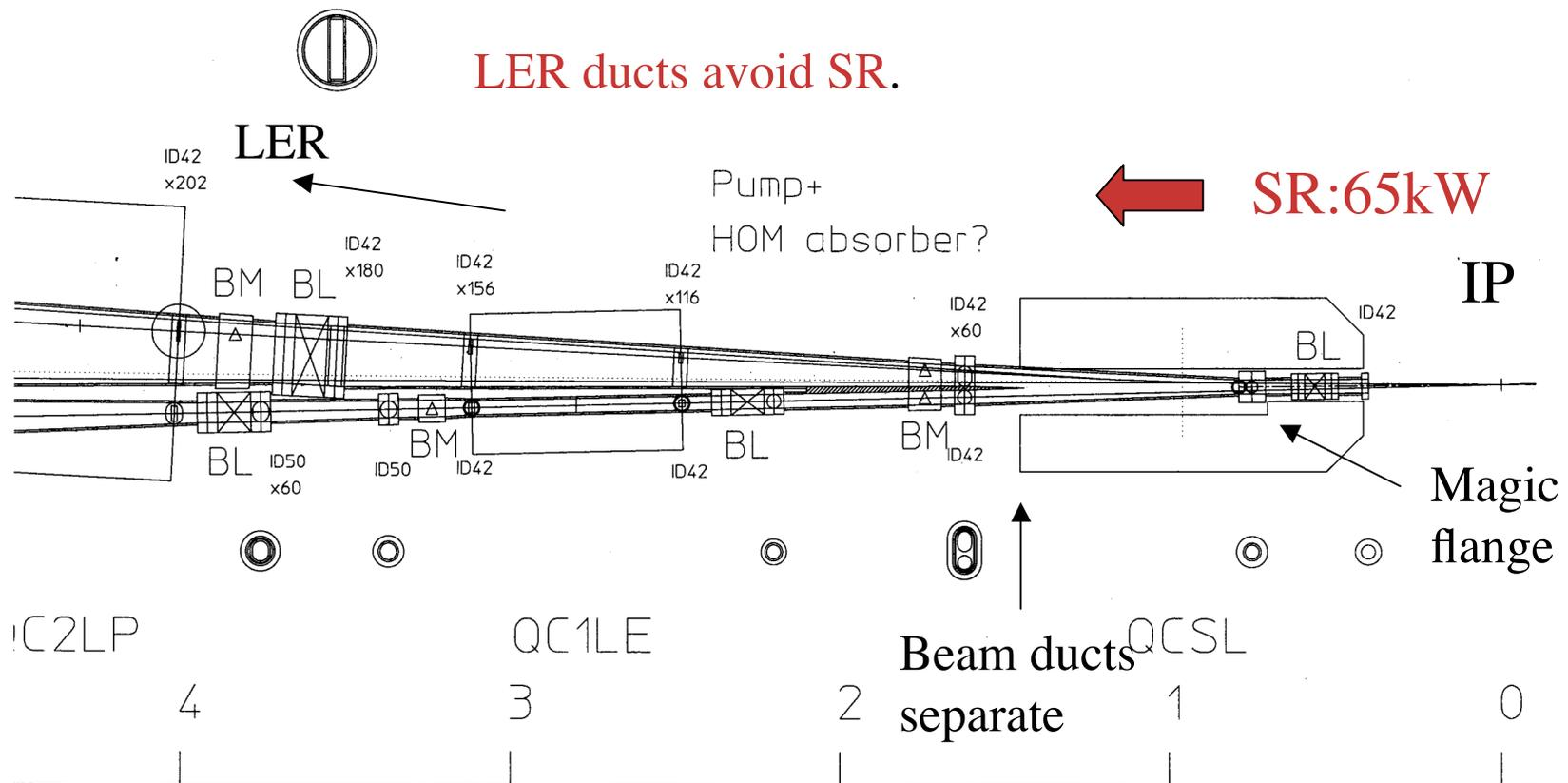
BM:Beam Position Monitor, BL:Bellows
