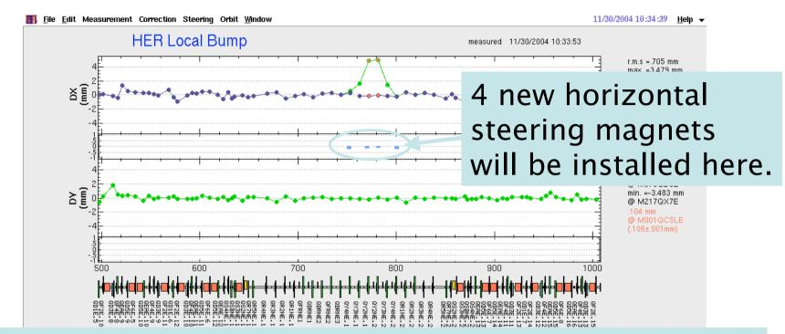
If  $\Delta x$  at crab cavity is measured to be +1 mm, create a -1 mm bump using these 4 steering magnets. (5 mm offset bump with 0.2 mrad kick angle possible)
