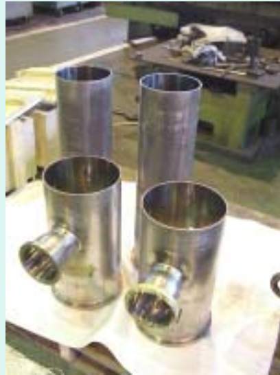
Beam Pipes were Fabricated by E.B.W.
