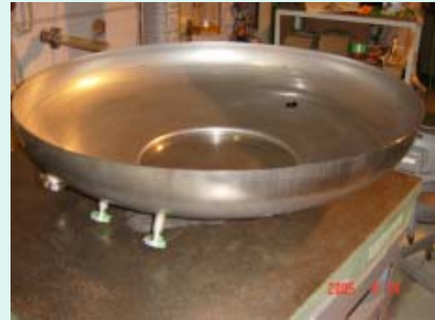
Helium Vessel for Large Beam Pipe
