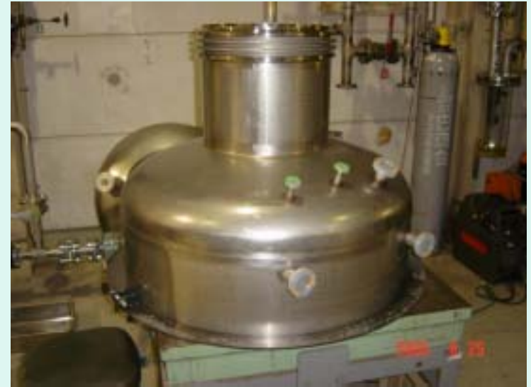
Helium Vessel for Small Beam Pipe
