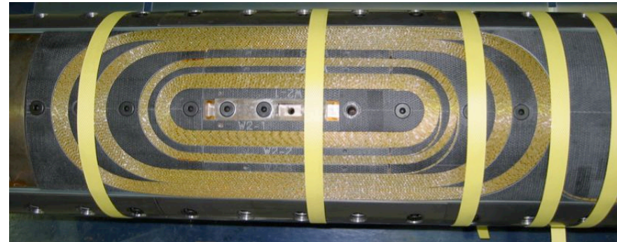
2nd layer coil after winding 1st layer coil
