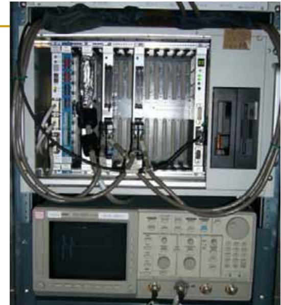
BPM DAQ system (VME + Oscilloscope with GPIB)
