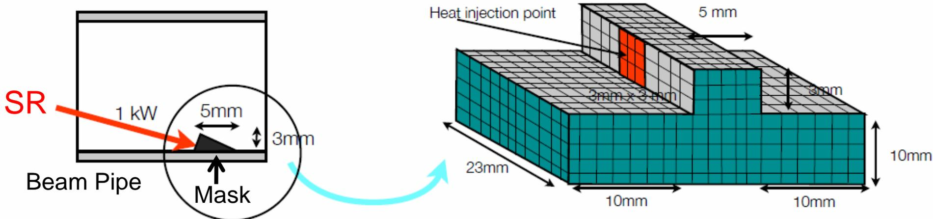
Material : copper is assumed (because of its good thermal conductivity)
