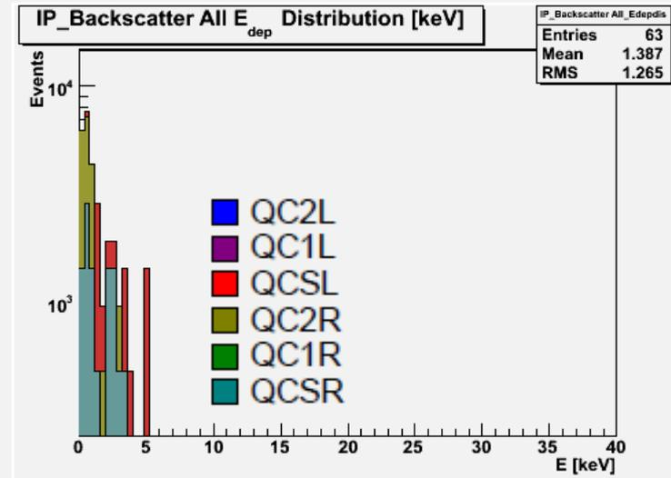
Back scattered particles in IR are caused by SR produced at QCSL
