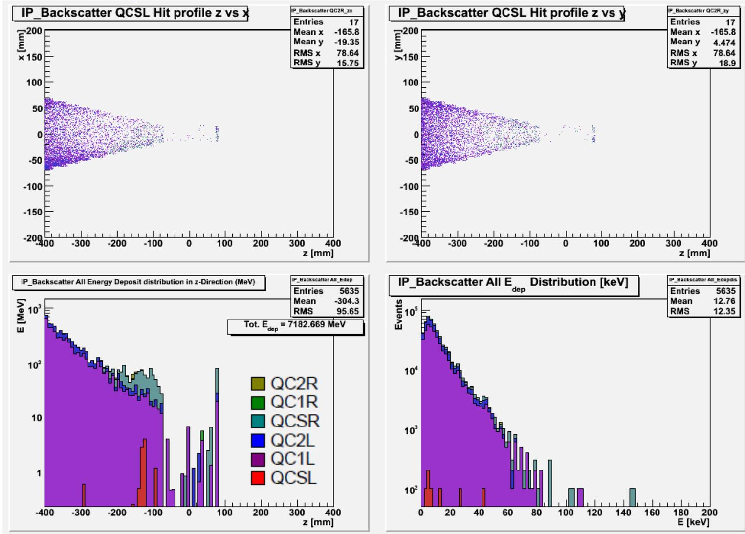
Back scattered particles in IR are caused by SR produced at QC1L & QCSR
