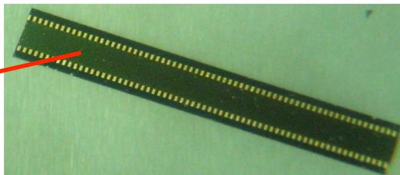
Fermionics InGaAs detector array. Also being used at CesrTA (with Cornell-developed mount and readout).
