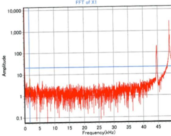
A betatron oscillation of a pilot bunch was successfully excited by PLL.
