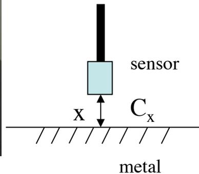
Gap detector developed at KEK.
