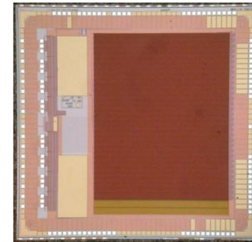
STURM ASIC for high-speed readout (G. Varner).
