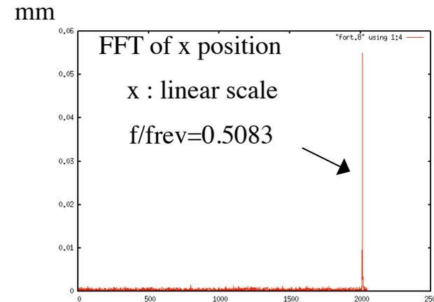
FFT of a gated signal measured by a turn by turn BPM
