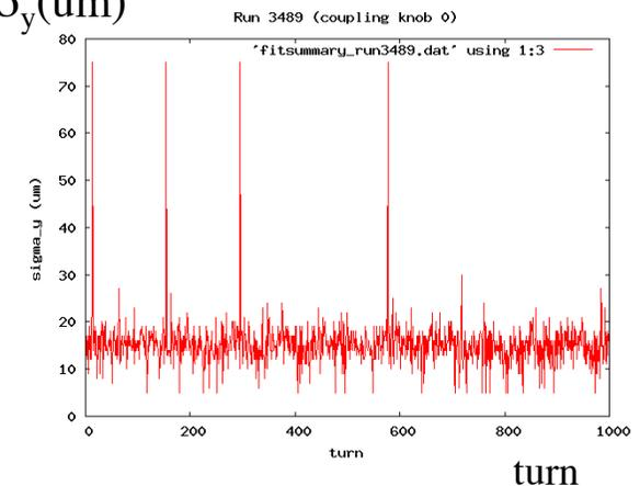
Turn-by-turn single-bunch measurements at CsrTA
