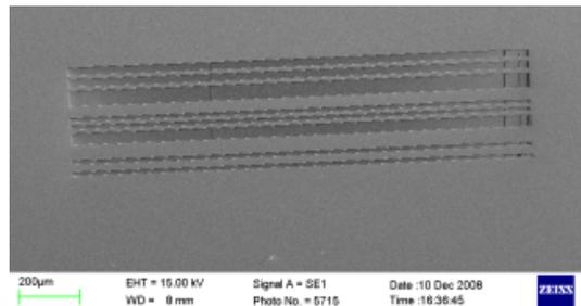
Uniformly Redundant Array (URA) for x-ray imaging being tested at CsrTA
