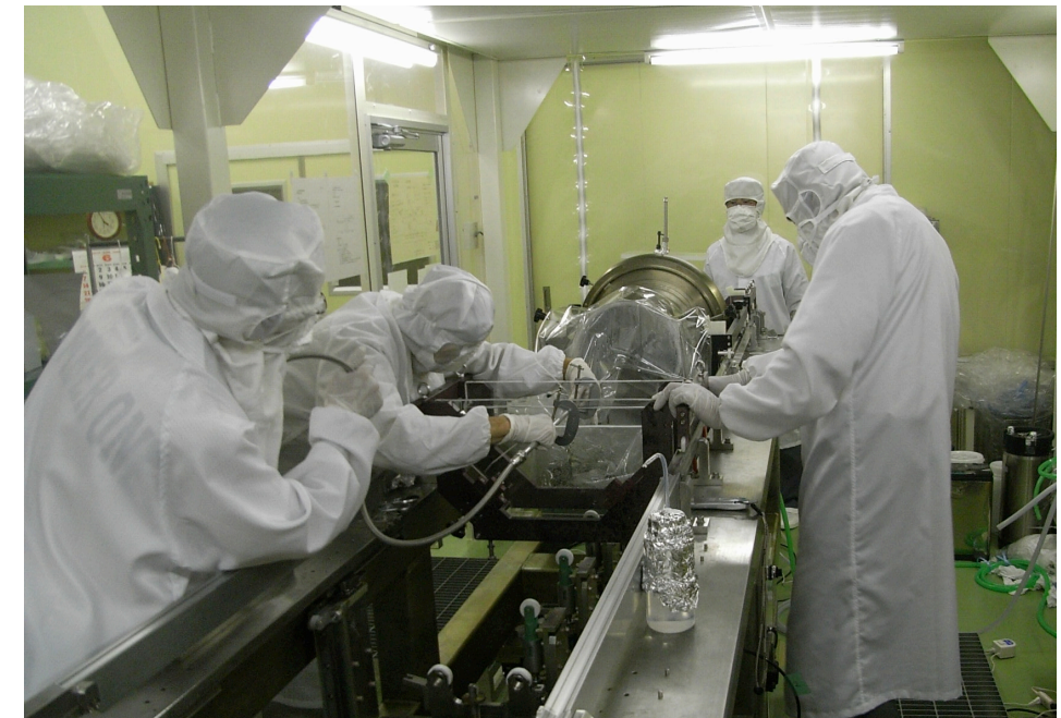
Rinsing a prototype cavity in a clean room
