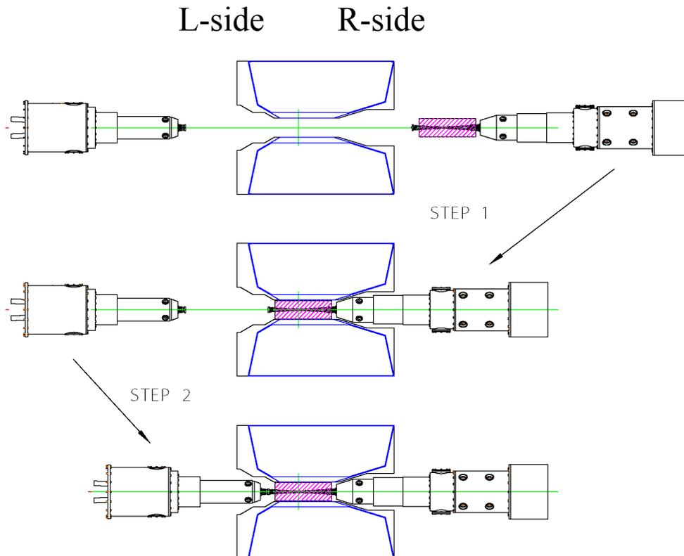
1. Connect IP chamber with SVD4 to the QCSR cryostat.
