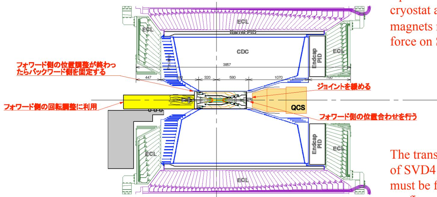
The transverse position of SVD4 forward end must be fixed in this configuration.
