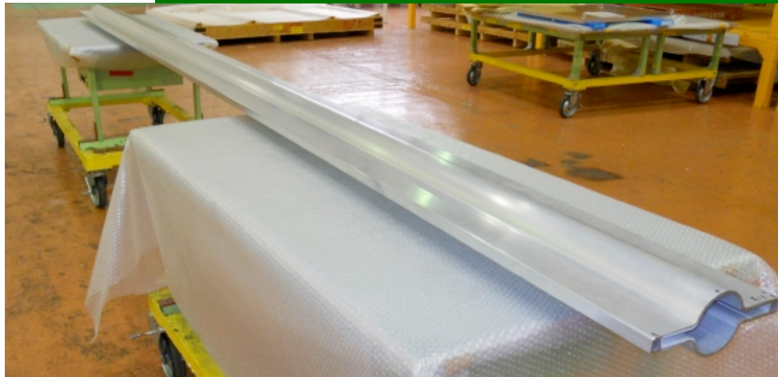
Aluminum beam pipe with antechambers (extrusion)
