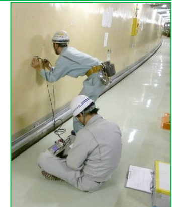
Measure Level by Hydrostatic water Level System (HLS)
