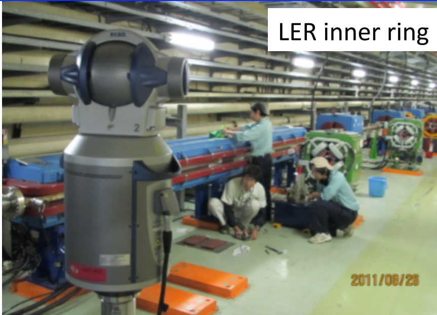
3. A) Survey for the new (longer) LER dipole magnets with laser tracker
