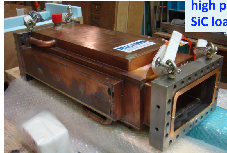
Copper waveguide with directional coupler
