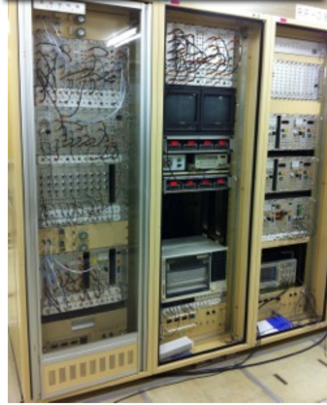
Present LLRF System of the KEBB (for one klystron)
