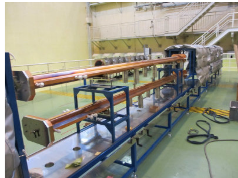
Baking station for long beam pipes.
