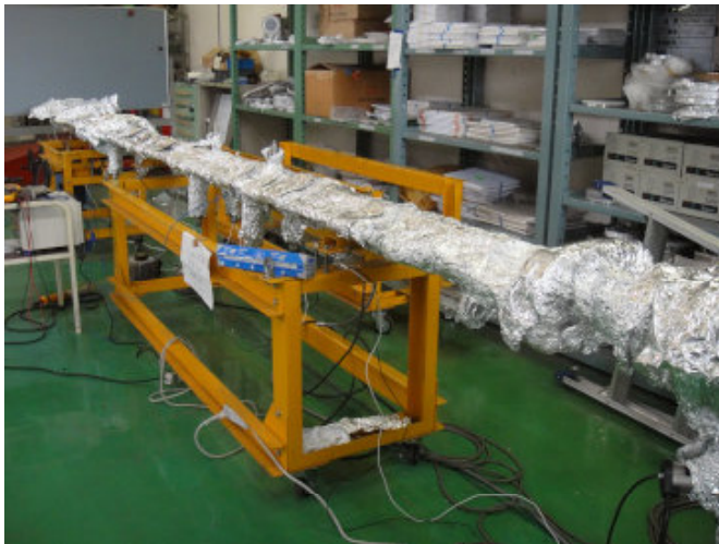
Conventional baking style with tape heaters and Al foils
