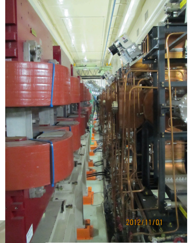
Six ARES cavities in D5 moved from HER to LER. HER wiggler magnets were installed close to the ARES.
