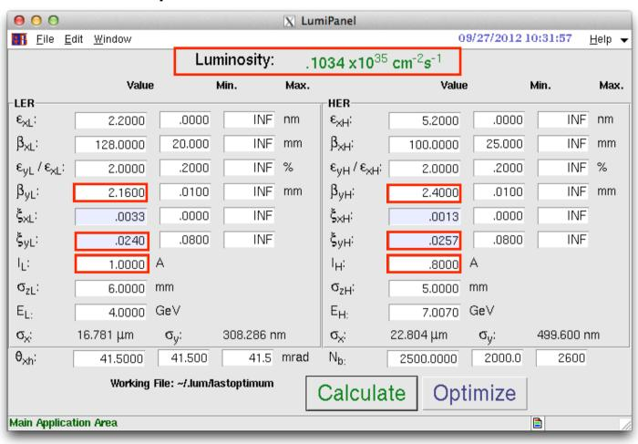
$\beta_x^*$ : x4,  $\beta_y^*$ : x8, coupling =2 %,  $\xi_y \sim 0.025$ ,  $I_{LER} = 1$  A. The effect of intra-beam scattering is decreased in LER.
