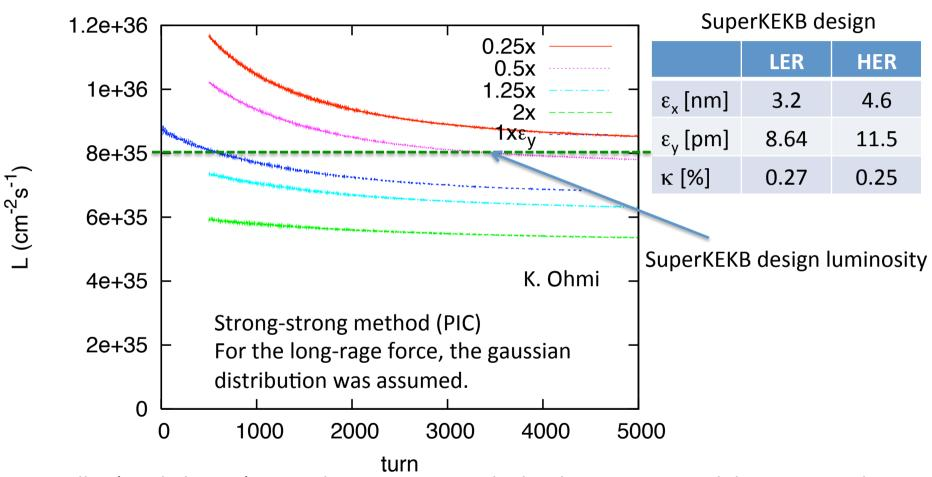
Smaller (single beam ) vertical emittance gives higher luminosity. Much lower vertical emittance than the design (about half) will be needed to achieve the design luminosity. A tentative target of x-y coupling w/o beam-beam is 0.15%.
