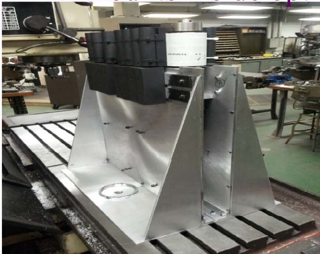
PMT mounts inside optics box
