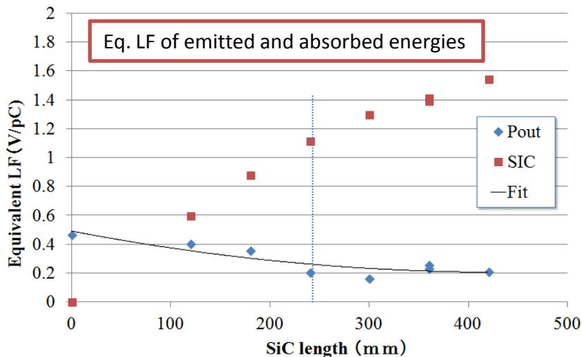
Additional SiC damper can absorb more energy as the length becomes longer. It also reduces SBP and LBP damper loads. In practice, HOM load of additional SiC damper has to be less than 30kW (1.1 V/pC). 240 mm damper is suitable for our cavities.
