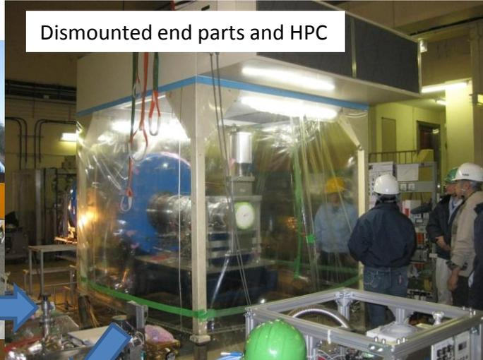
High pressure water jet in cavity cell
