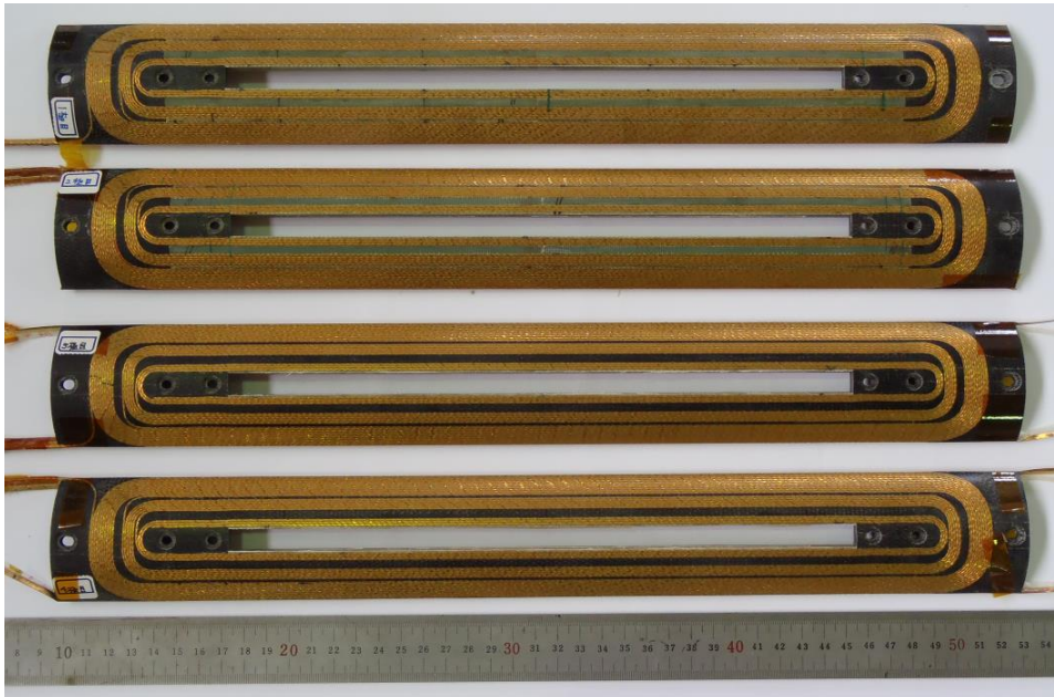
Four double layer coils
