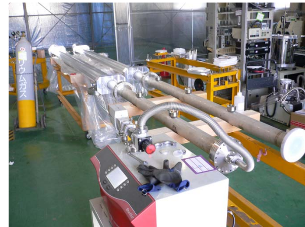
Leakage test before installation
