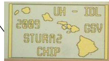
STURM ASIC for high-speed readout (G. Varner).
