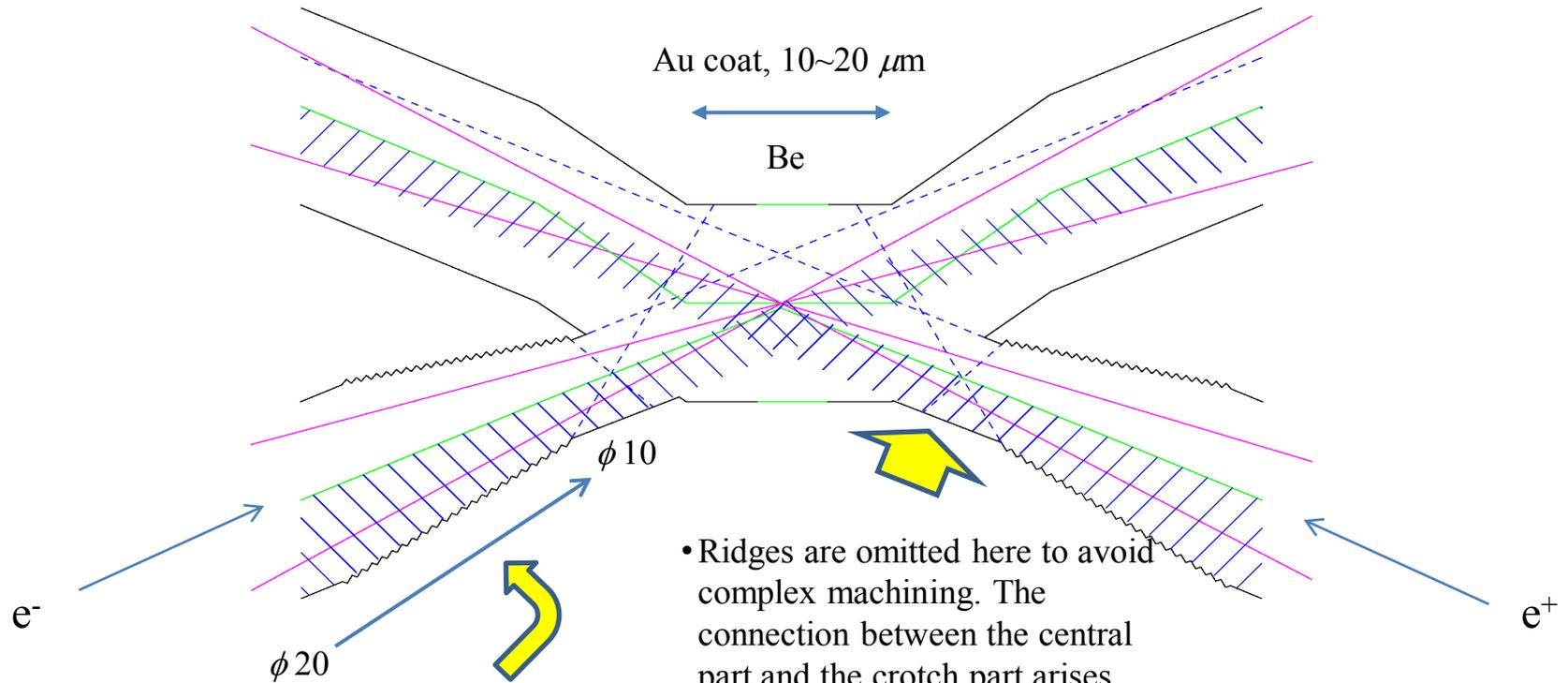
Taper: to reduce the number of photons entering into the central part
