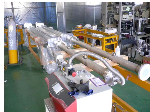
Leakage test before installation
