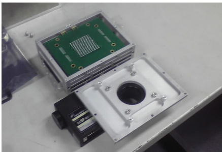
Si deep-pixel detectors and spectrometers for the X-ray monitor. (SLAC)
