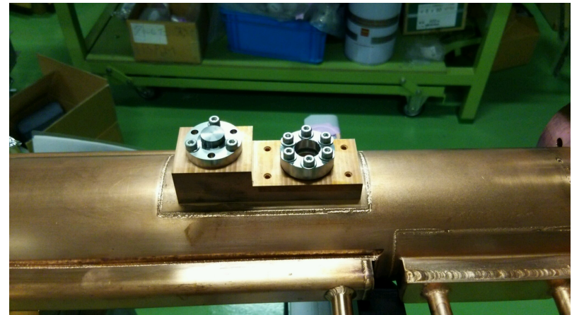
Test fit of LABM extraction mirror (left) and extraction window (right) on IR beam pipe.
