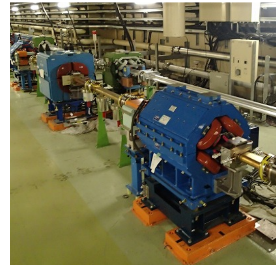
Magnet installation in the mid-arc sections
