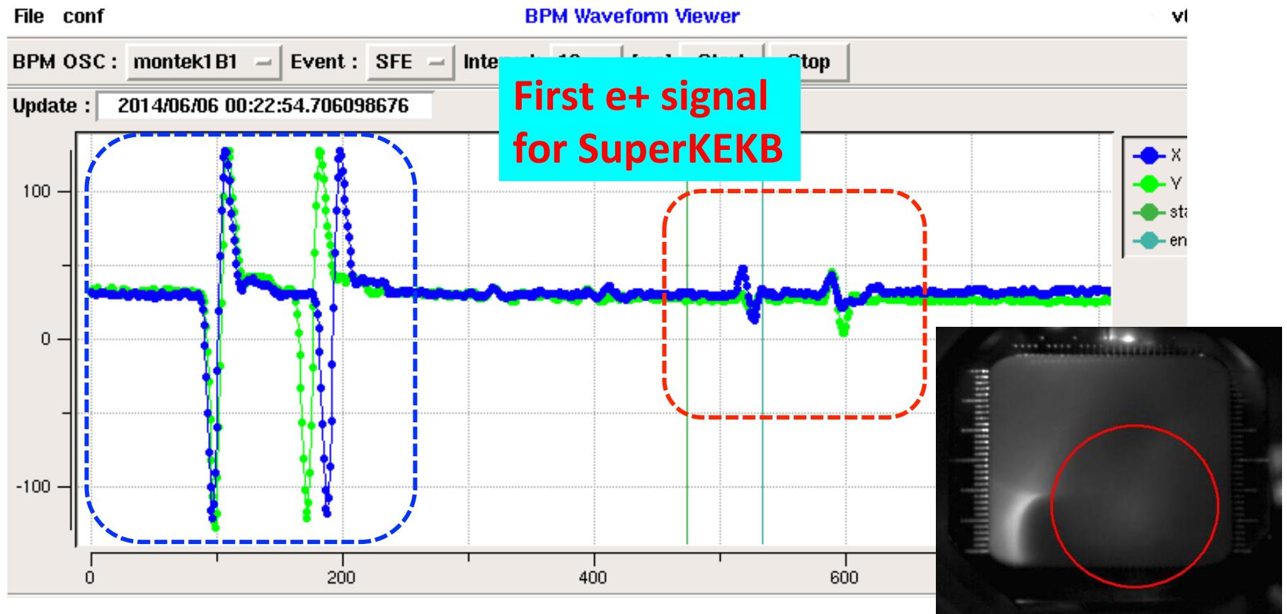
BPM: SP\_15\_T in front of target negative charged particles (e- beam) give (-)(+) bipolar signal
