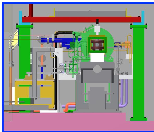
Radiation shield structure (**200-mm thick iron**)
