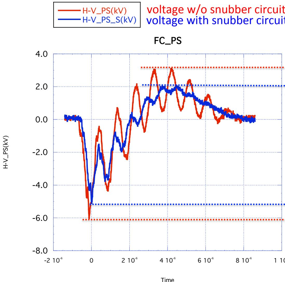
Before start of 2014 autumn run, we removed snubber circuit for convenience of future FC exchange work. It should triggered the cable accident.
