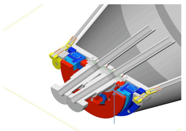
These components rotate to catch the bellows flange.
