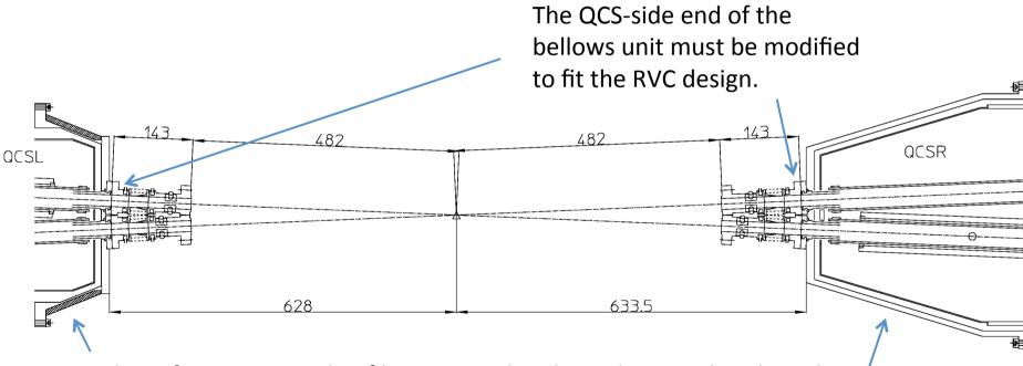
These front caps made of heavy metal and stainless steal replace the original caps when RVCs are installed. The design of their front face must be done along with the design of RVC.
