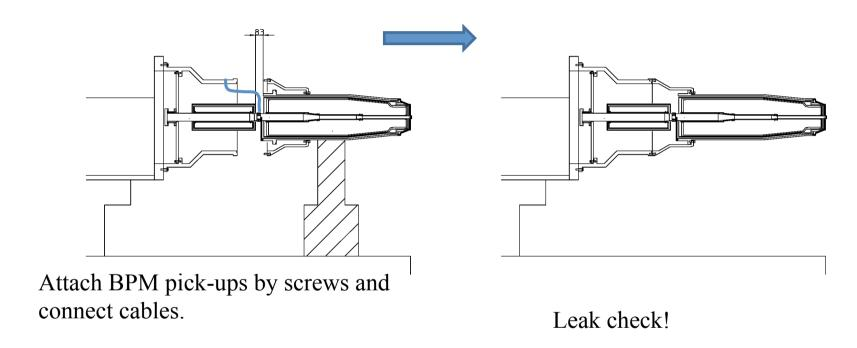
This installation work seems very delicate. In preparing assist tools, necessary conditions must be discussed and be clarified.
