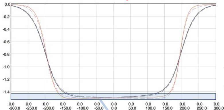
Belle II solenoid field looks sensitive to coil shift compared with Belle.
