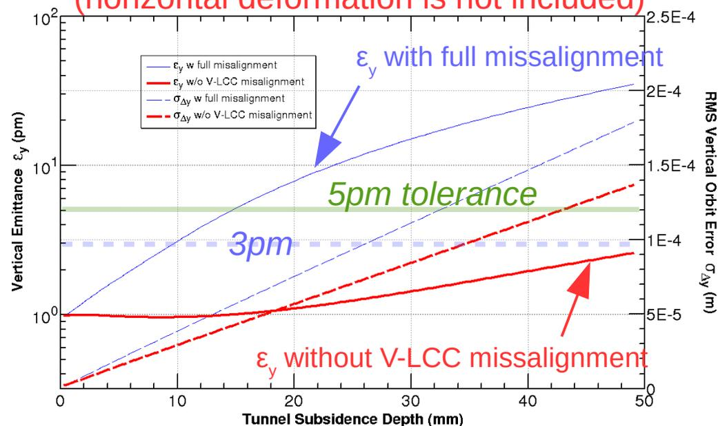
Tunnel subsidence model is generated from latest measurement with LPF( $\lambda_{cut} \sim 100\text{m}$ ).
