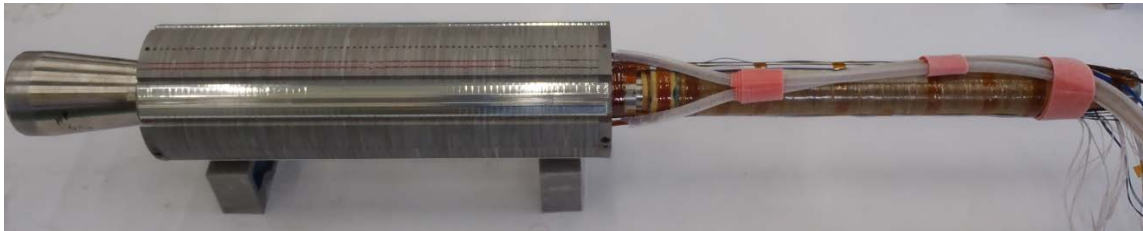
QC1LP leak field cancel magnet
