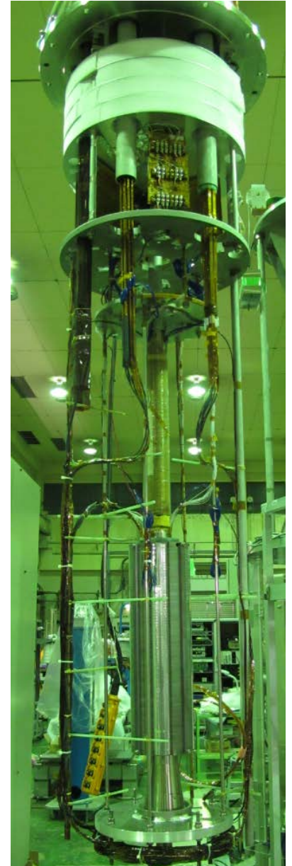
QC1LP leak field cancel magnet
