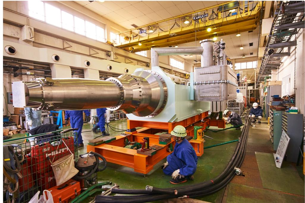
QCSL magnet cryostat was set in the Super. Cryo. Vac. Experimental Laboratory at Dec. 25 and 26, 2015.
