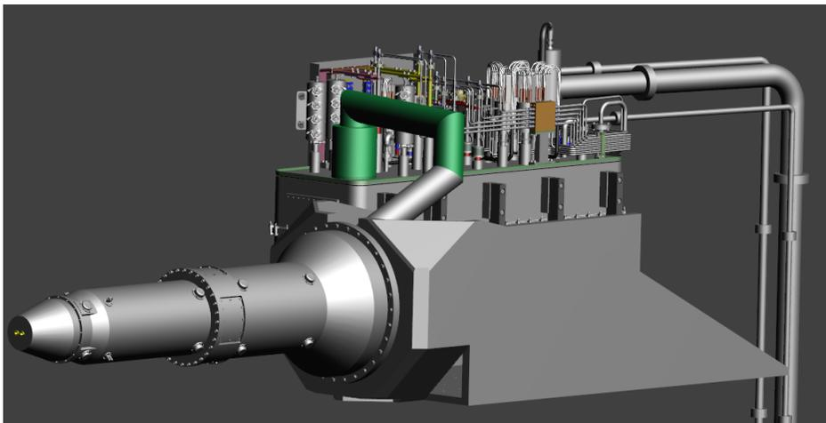
Drawing of QCSR cryostat. QCSR is now under fabrication at Mitsubishi, and will be completed this autumn.
