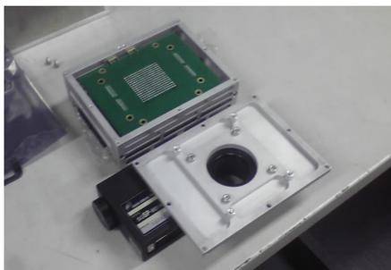
Si deep-pixel detectors and spectrometers for the X-ray monitor. (SLAC)
