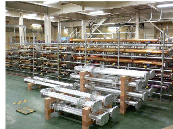
Copper and Aluminum beam pipes after baking and TiN coating. They are temporary stocked in Oho B4 until moved to tunnel or other stock houses.
