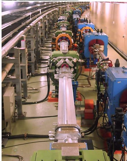
Replace beam pipes with TiN-coated antechamber-type ones
