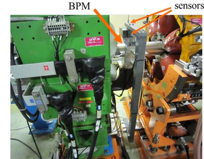
Displacement sensor near a rotatable sextupole magnet.
