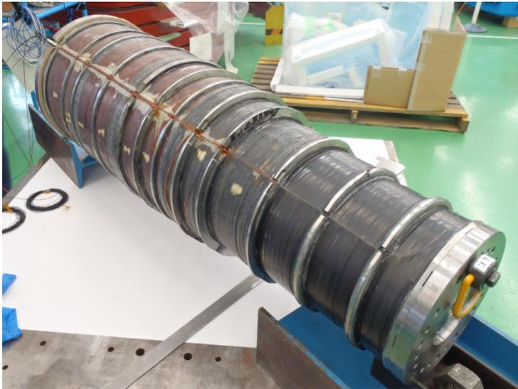
Completed ESL compensation solenoid. The solenoid was divided into 12 small solenoids.
