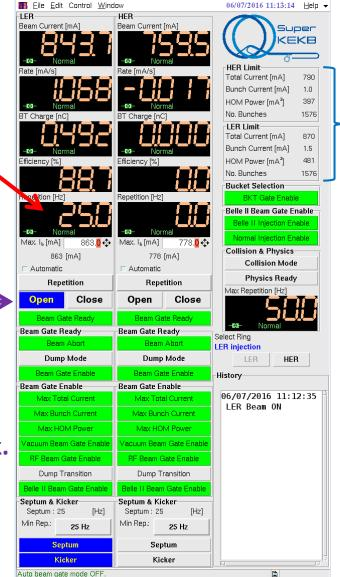
Current Limit Setting Injection is stopped (Beam Gate is closed) when the beam current exceed these limits.
