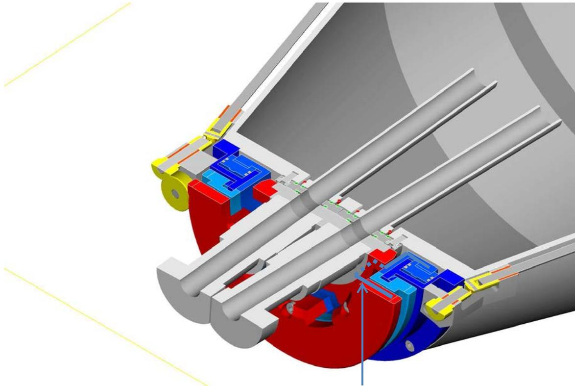
These components rotate to catch the bellows flange.
