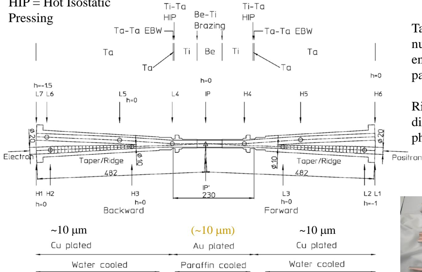
Only taper parts are exposed to direct synchrotron radiation from the last bend.
