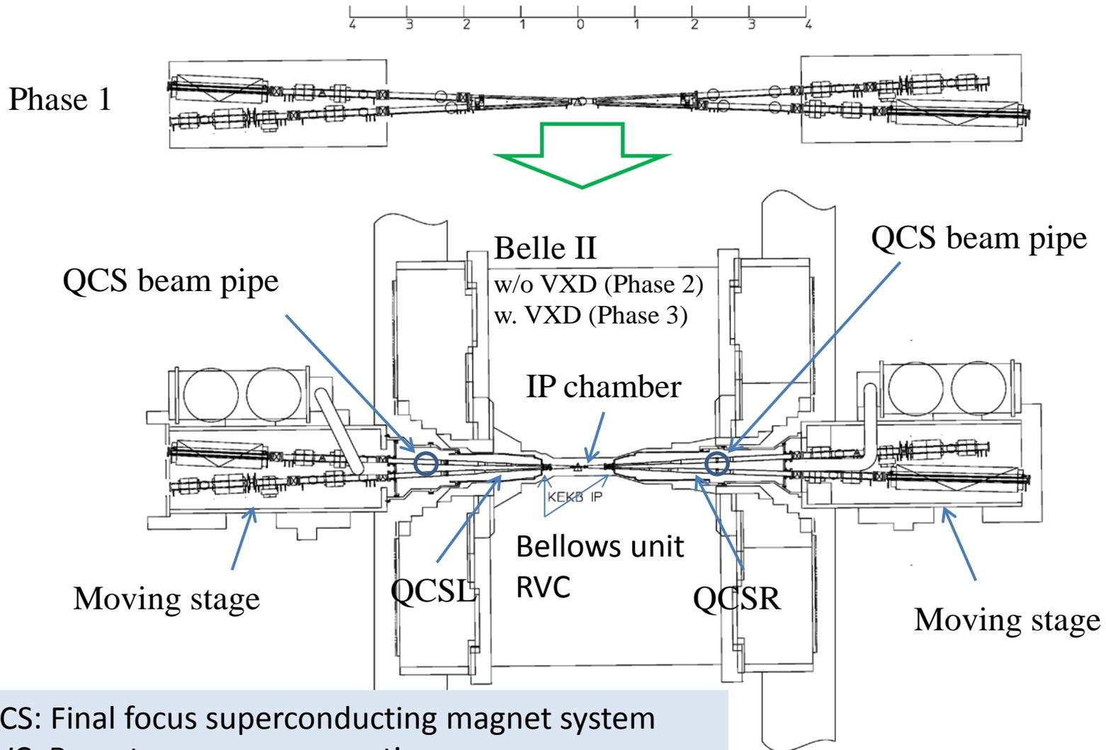
QCS: Final focus superconducting magnet system
