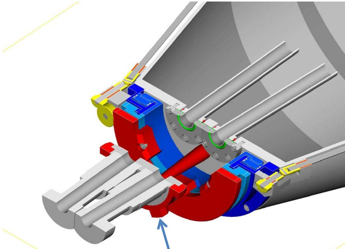
Two bellows units are attached to a single flange with a retainer.
