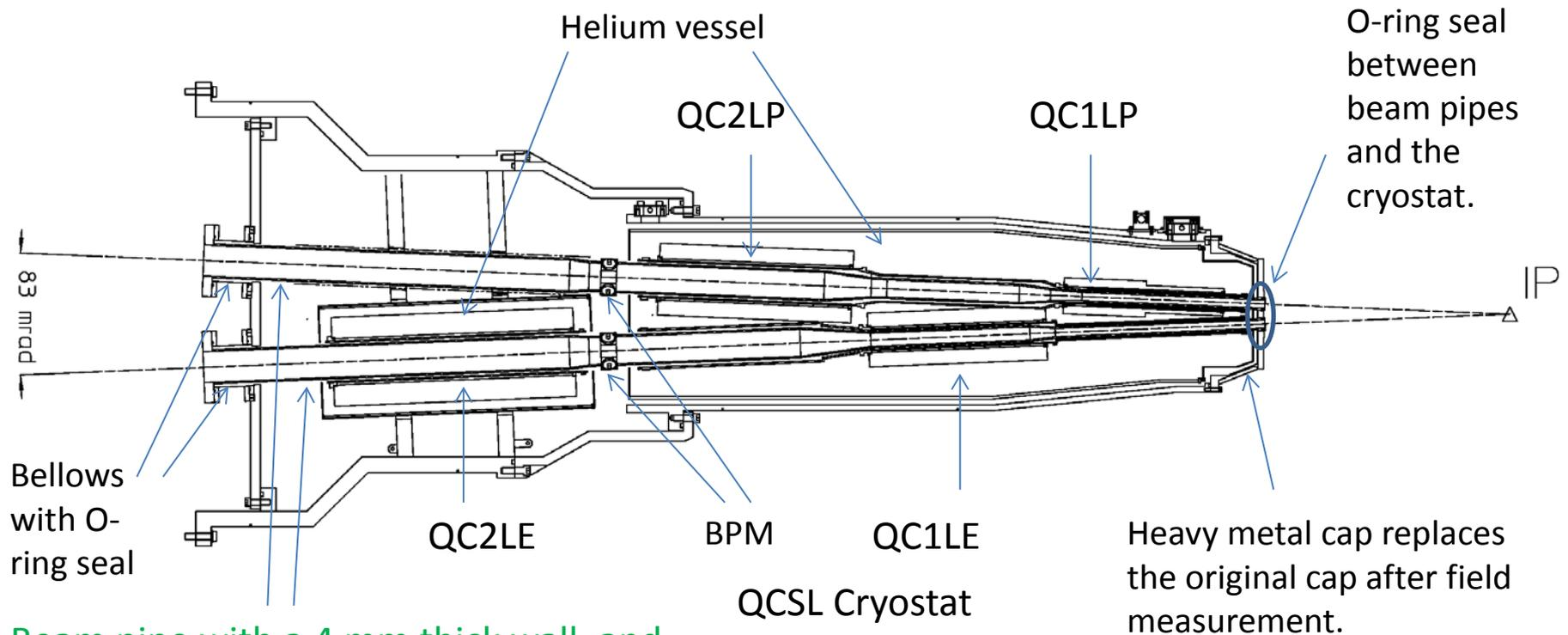
Beam pipe with a 4 mm thick wall, and with water cooling channels therein.
