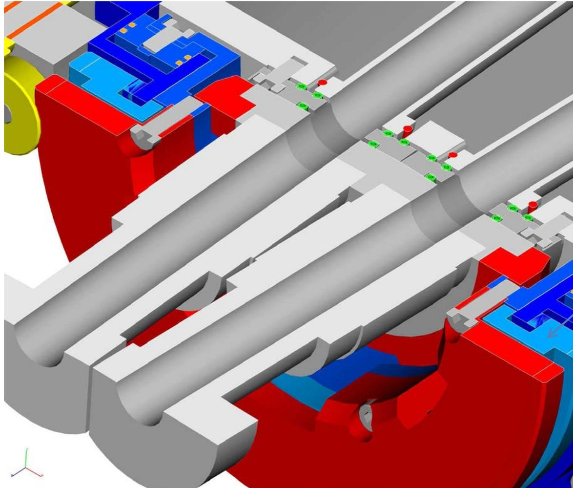
This large screw nut turns to lock the mechanism.
